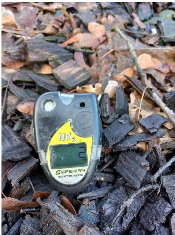
Ammoniakmetingen boven biobed. (concentratie is 2 tot 3 ppm)
