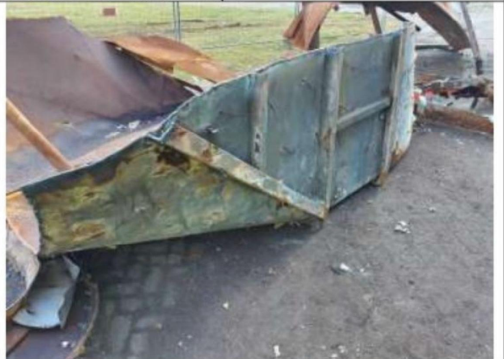
Description photo: 12-3-2021 parts off separation between FGD and Precips
